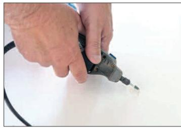
Use a dremel tool fitted with a burr bit.
