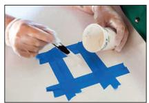
Use a mixing stick to run the gelcoat into the crack.
